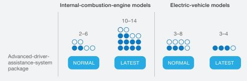
Electronic control units per vehicle by engine type and driver assistance package, range
